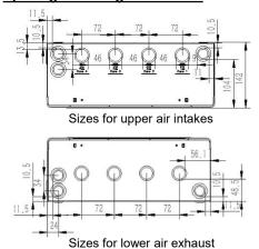
The detector is fixed on the wall using expansion bolts (using M4 screws). The spacing between the mounting holes is 312mm. The **sampling pipe\*** that is compatible with the detector shall have an outer diameter of 25mm and an inner diameter generally of 21mm. Other external dimensions and detailed installation dimensions are shown in the diagrams.
